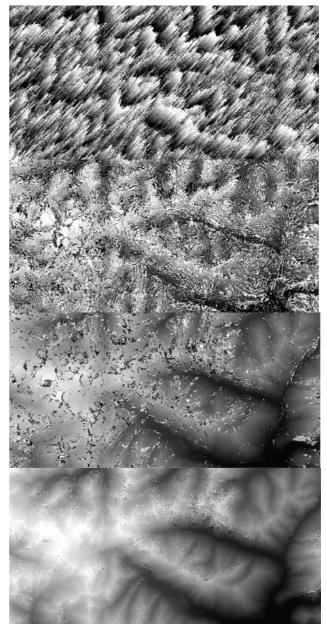
Fig. 5. Digital Elevation Model of Sterzing, Italy, reconstructed from multi-geometry SRTM data using a maximum likelihood approach. Size: 30 km by 15 km. Top to Bottom: increasing accuracy with increasing number of observations: 1, 2, 4, 4 observations plus external reference
