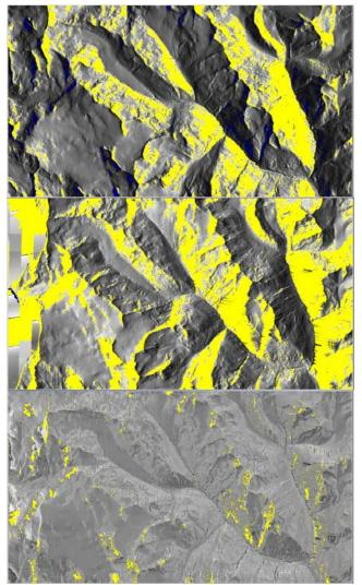
Fig. 6. Simulated shadow and layover areas (yellow) in the steep Ötztal mountains (Austria) for  $41^{\circ}$  incidence angle descending (top),  $30^{\circ}$  incidence angle ascending (mid) and a combination of both (middle).
