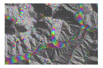
Fig. 2. Geocoded SRTM X-SAR interferometric phase image of Nanga Parbat (NP). The phase is shown in cyclic false colors, the luminance taken from the SAR intensity. One fringe corresponds to app. 175 meters elevation difference.
